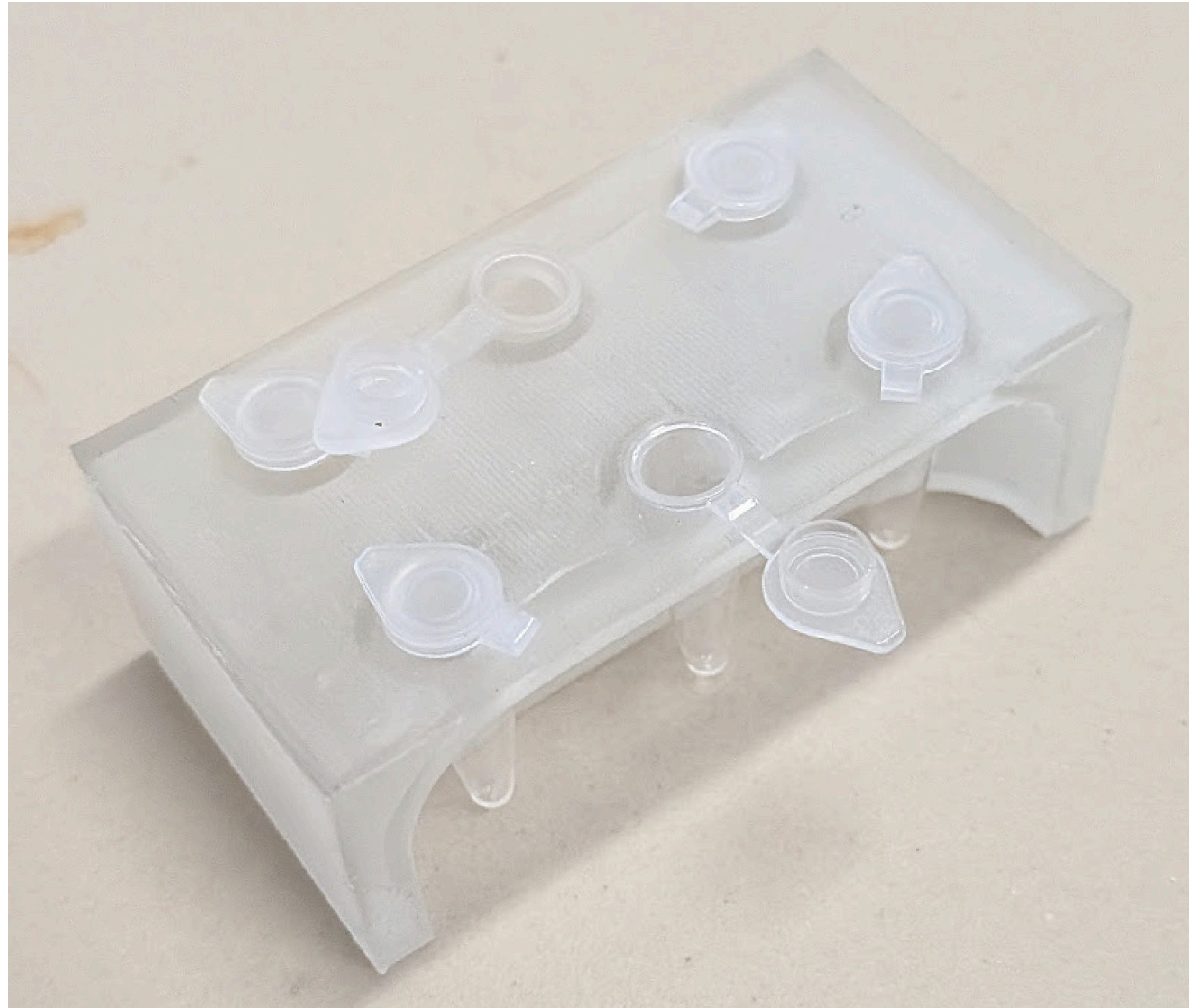
Figure 18: The Eppendorf holder I designed for the lab.
