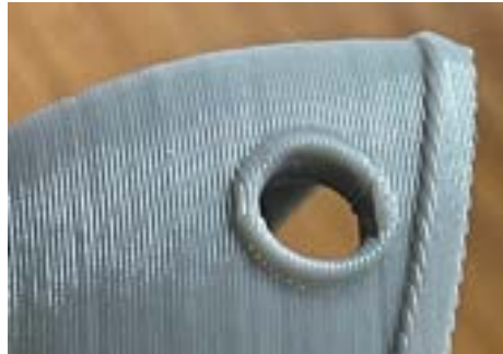
Figure 8: A closer look at the layers in the 3D print.
