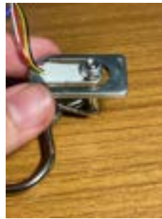
(b) Load cell with a protected strain gauge.
