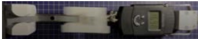
Figure 21: The breaking of a random measurement, in this case at 16,98 kg for a 200^\circ , 0.25 mm bar.
