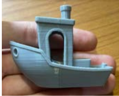
Figure 7: 3D Printed object with the same settings as in the diagram, using a 0.2\text{mm} layer height at 220^{\circ}\text{C} and a 0.4 .
