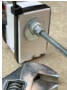
(a) Washer and double nuts that are tightened to apply force
