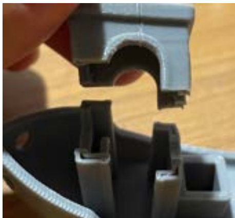
Figure 2: A 3D printed boat that broke parallel to the printing lines. Own source.
